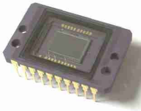
Monochromer, Progressive Scan 2/3"-CCD Bildsensor Sony ICX285AL
