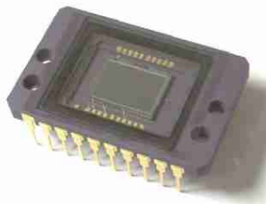
Monochromer, Progressive Scan 2/3"-CCD Bildsensor Sony ICX285AL
